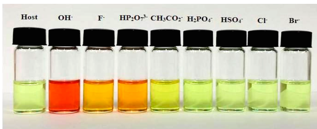
Figure 5. Color changes of receptor 1 at 100 \mu\text{M} in DMSO when treated with 70 equiv of various anions.
